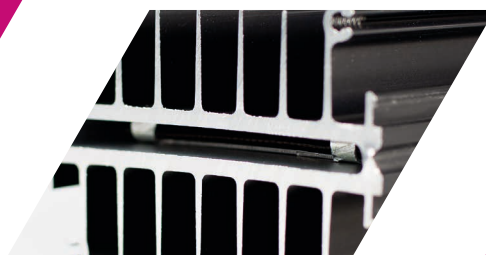
PTC heating element for self-regulation (current depending on temperature of heater).
